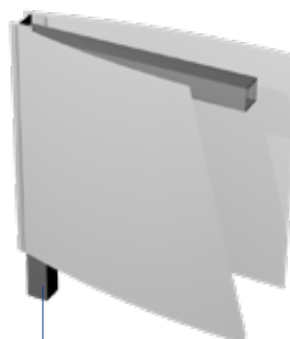
Aluminium or steel profile 60 x 60 x 4mm Aluminium- eller stålprofil 60 x 60 x 4mm
